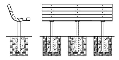
ALL SEAT BRACKETS AND FOOT MOUNTING BRACKETS ARE 3/8" X 4" STEEL BAR STOCK
