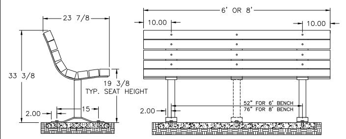
FRAMES SHOULD BE ANCHORED TO A CONCRETE PAD PROVIDED BY THE CUSTOMER
